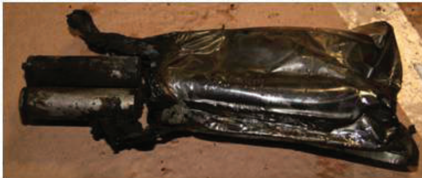
Figure 5. A non-compliant laptop battery ordered online and sent by airmail, which caught fire shortly after being unloaded from a passenger aircraft at London Heathrow Airport
