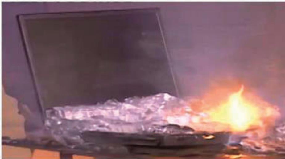
Figure 5.6. A demonstration of the effect of applying ice to a burning lap top (courtesy of the Federal Aviation Administration)
