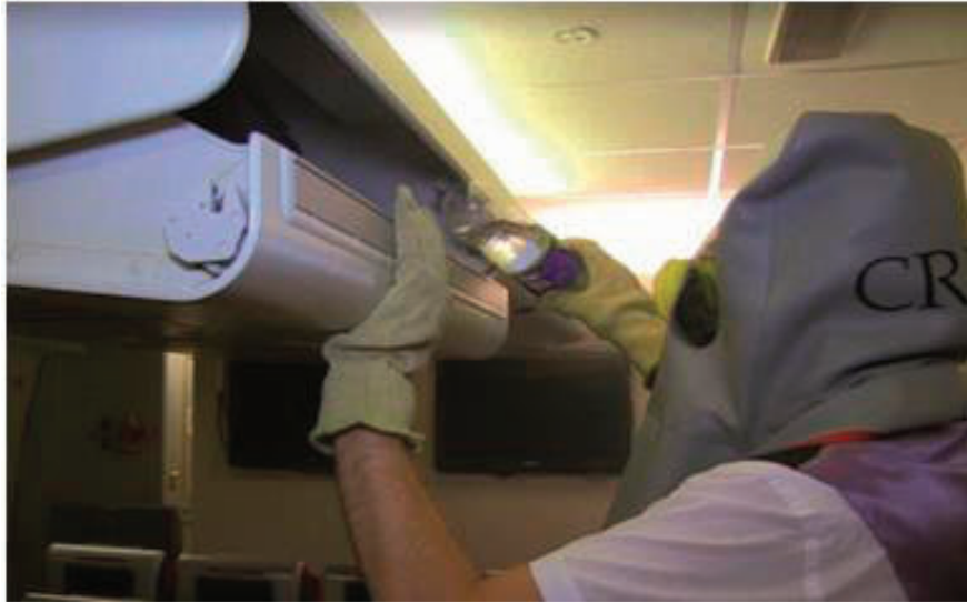
Figure 5.5. Applying water to a lap top computer without removing it from an overhead locker Note - Liquid may turn to steam when applied to the hot battery.
