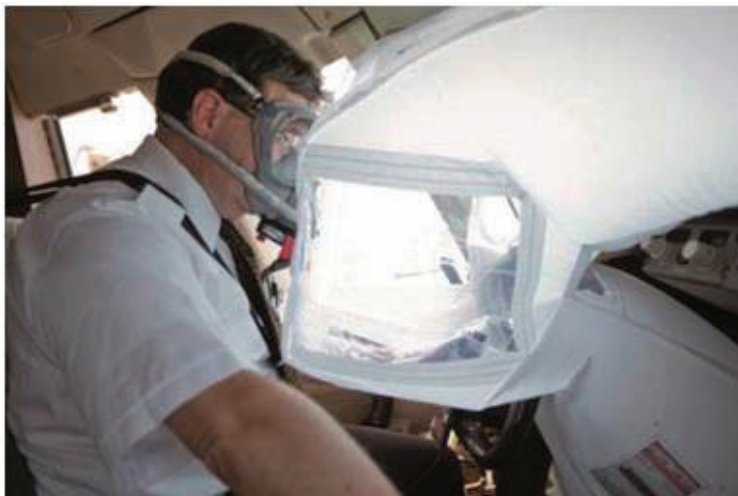
Figure 6.5. A smoke displacement system (EVAS - Enhanced Vision Assurance System)
