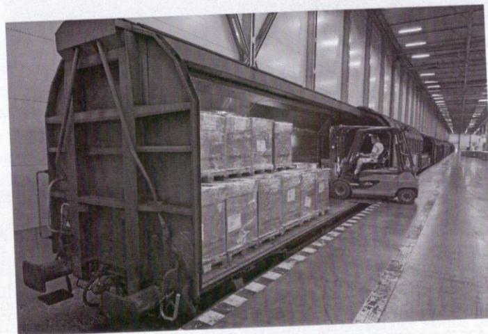
Figure 2.22 Covered wagon being unloaded by a forklift. (From Port of Gothenburg.)
