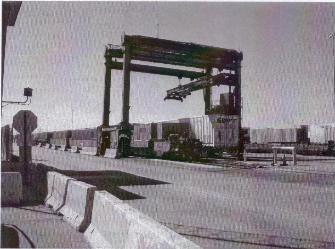
Figure 2.11 Rubber-tired gantry crane. (From Rickard Bergqvist and Jason Monios.)
