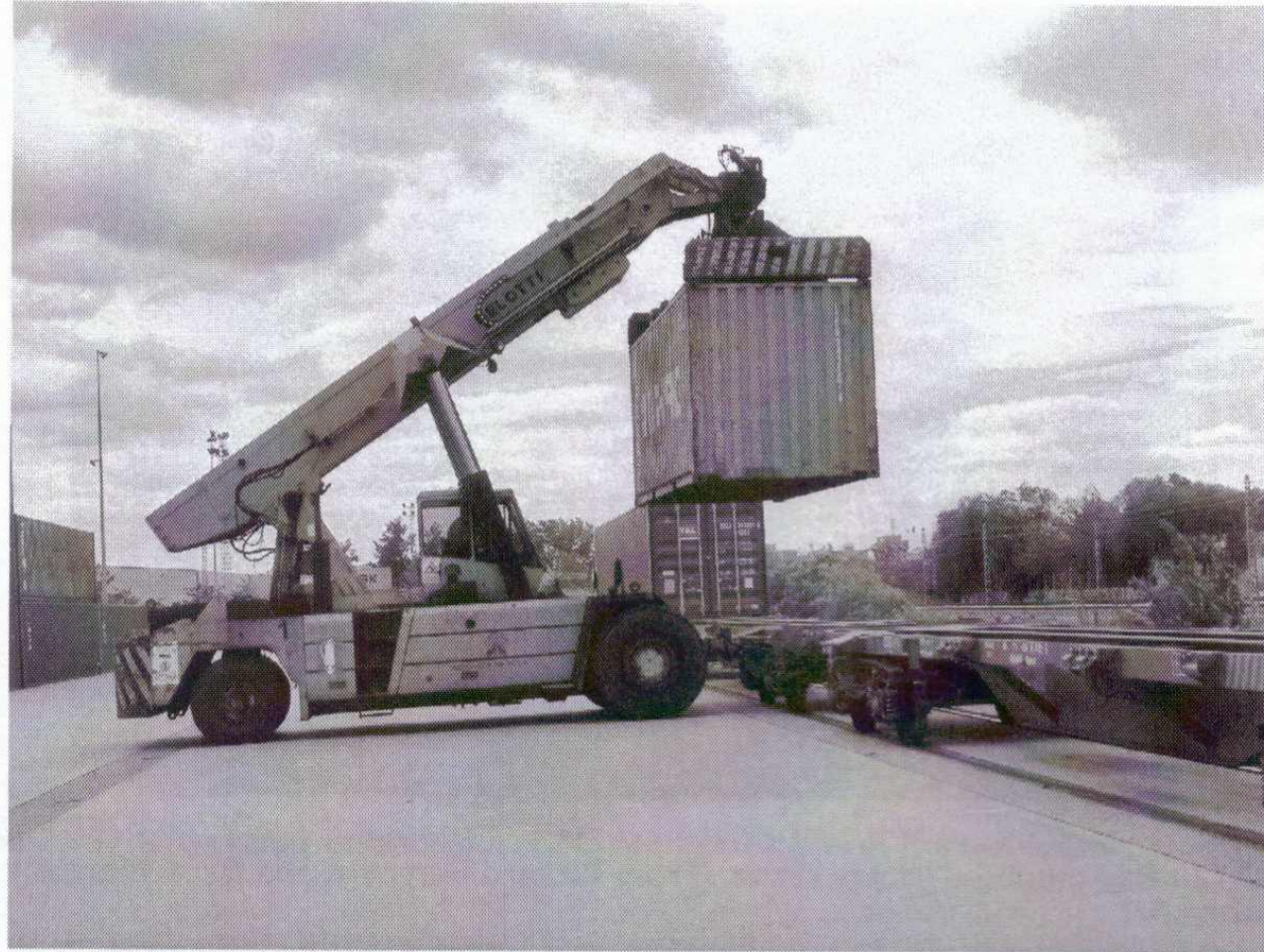
Figure 2.10 Reach stacker loading a container onto a train. (From Rickard Bergqvist and Jason Monios.)
