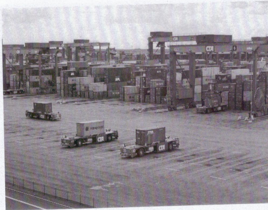
Figure 2.15 AGVs in operation at a port container terminal. (From © Henrik Jesser BY 3.0] via Wikimedia Commons.)
