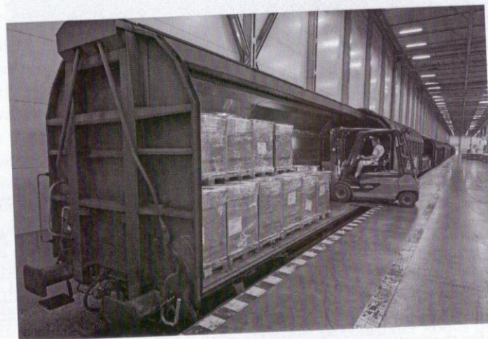
Figure 2.22 Covered wagon being unloaded by a forklift. (From Port of Gothenburg.)
