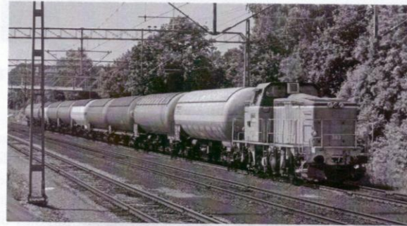
Figure 2.24 Tank wagons. (From Port of Gothenburg.)
