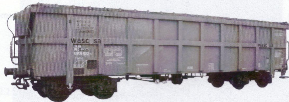
Figure 2.20 Open wagon with tarpaulin cover. (From Wascosa.)
