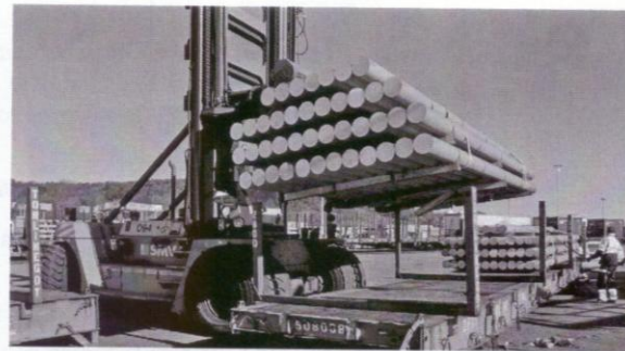
Figure 2.25 Flat wagon with uprights for hauling general cargo such as steel pipes. (From Port of Gothenburg.)
