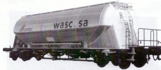
Figure 2.23 Powder wagon. (From Wascosa.)
