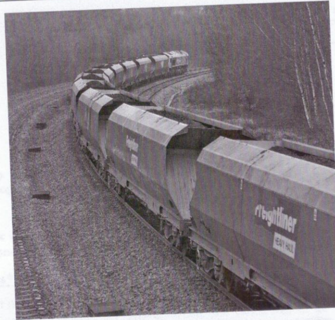
Figure 2.21 Open wagon. (From © Phil Sangwell [CC BY 2.0] via Wikimedia Commons.)
